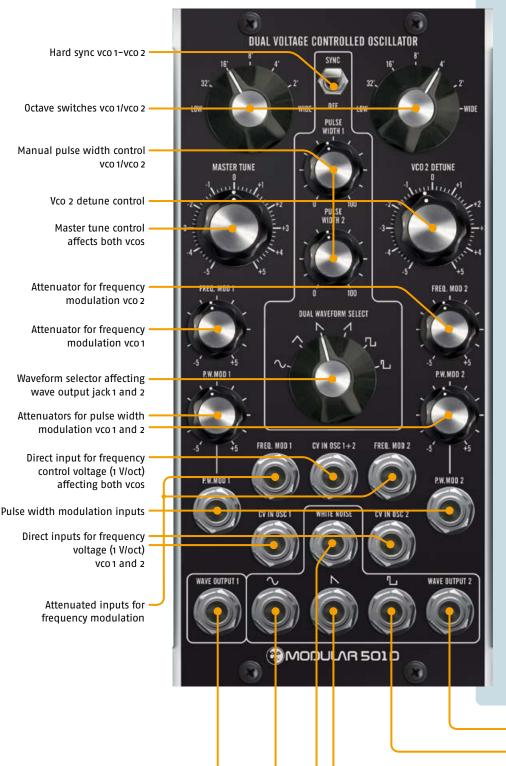
The M 501D **DUAL OSCILLATOR MODULE** combines two voltage controlled oscillator circuits in one double-width unit. The two oscillator halves enter a symbiosis in that they share some controls which affect both while other functions are individual to each oscillator.
