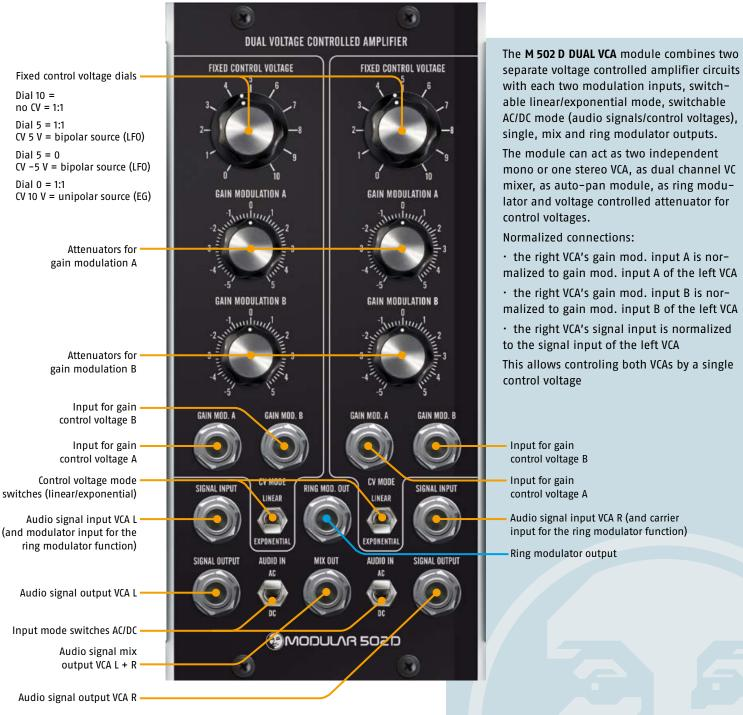
The module can act as two independent mono or one stereo VCA, as dual channel VC mixer, as auto-pan module, as ring modulator and voltage controlled attenuator for
