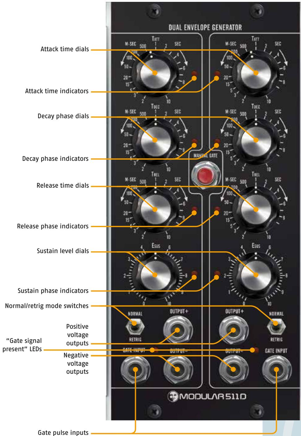
The 511D **DUAL ENVELOPE GENERATOR** module in typical ADSR-Style with four parameters: attack time, decay time, release time and sustain level.
