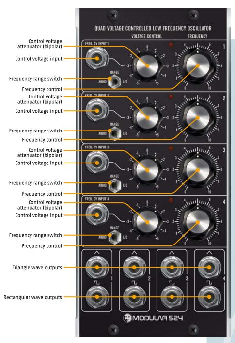
The M 524 **QUAD LOW FREQUENCY OSCILLATOR** module combines four voltage controlled low frequency oscillators.
