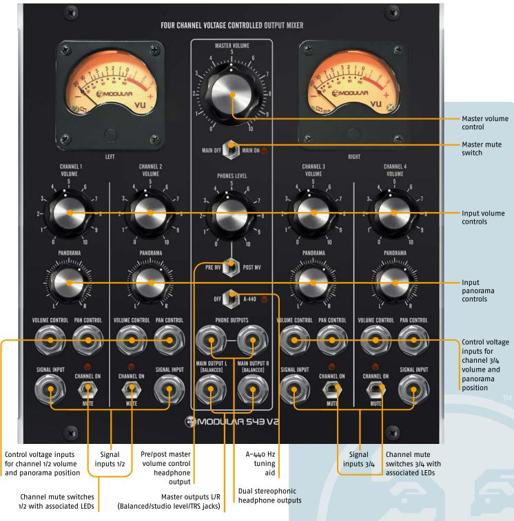
Four-channel master mixer for audio signals and control voltages with master-level control, channel on/off switches with status-LEDs as well as independent voltage controllable input volumes and panorama positions. Master volume control with dual stereo headphone outputs (switchable pre/post master
