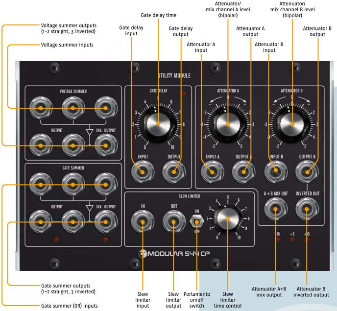
The **M 544 CP UTILITY MODULE** incorporates a couple of useful control voltage and logic functions in a CP sized module (4 units wide):
