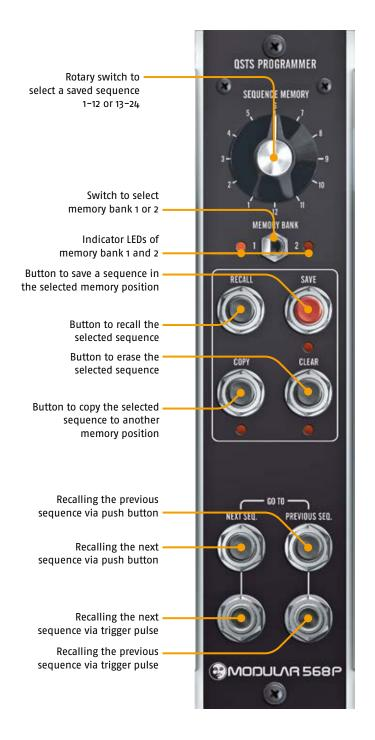
The M568P programmer module is an extension to the M568 Quad Sequential Trigger Source. Now 2 x 12 sequences/sequence-combinations can be saved to memory for later recall.
