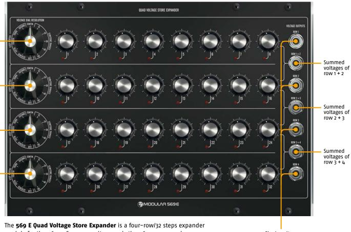
The **569 E Quad Voltage Store Expander** is a four-row/32 steps expander module for the 569 v2 Sequencer. It expands the 569 sequencer by 4 x 8 control voltage dials of which two rows can be combined to sum their corresponding output voltages.
