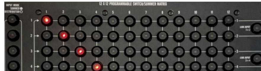
INPUTS 1 to 4 are „DISTRIBUTED“ to OUTPUTS 1 to 4
